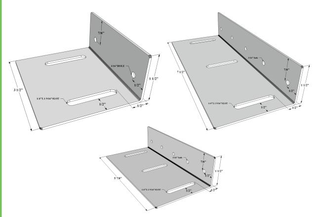
The deflection clips are used to allow a 1.5" (0.75" in each direction) deflection at the top of the wall.
